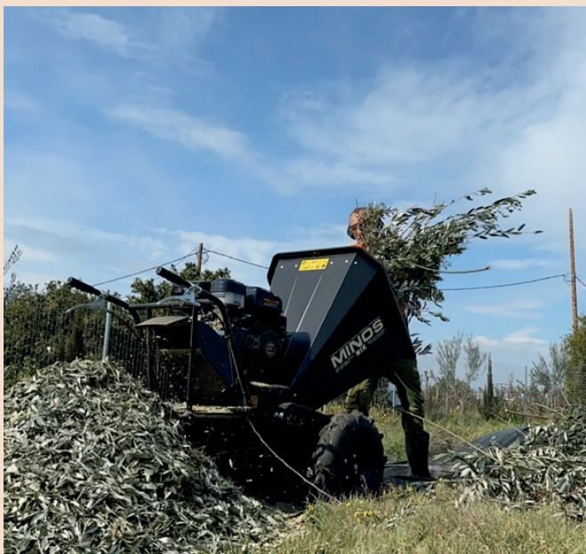
Figure 11: Left image: Shredding branches with a dedicated wood shredder allows placing the wood-chips directly under the trees where they are most needed. Right image: Mulching Cover crop and branches with the tractor is more efficient but the mulch is left between the rows.
